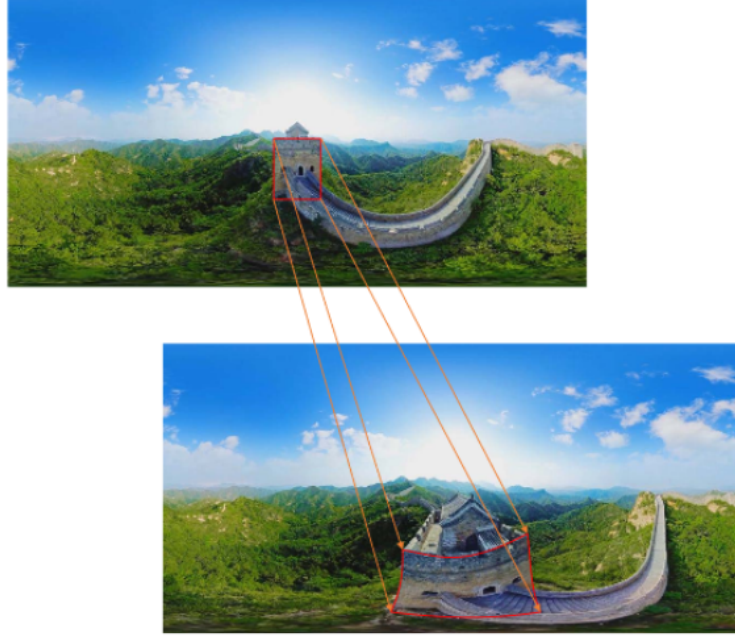
Figure 6: How 3D translation can deform a frame significantly with ERP [6]
